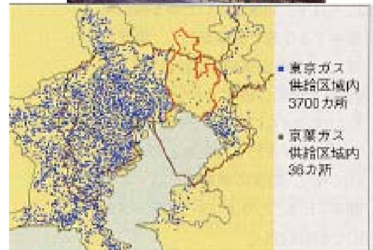
P.101 Fig.1(a) <Location of earthquake sensors deployed by TOKYO GAS Co., Ltd. >
