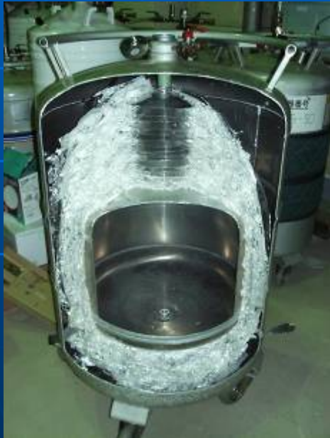
Cut-away view of a liquid helium vessel
